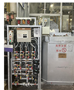
Holding furnaces for storing molten metal equipped hydrogen burners
