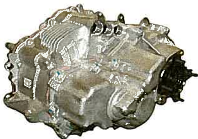
Photo 7 Appearance of Unit with Built-In Rear Motor and Differential Gear
