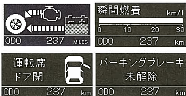
Photo 10 Display Example of Row of Three Instruments and Multi Display (Some Japanese Specifications Shown)
