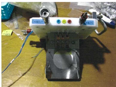
Fig. 2 Developed Temperature-Controlling Tool for Neutron Diffraction
