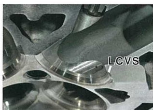
Fig. 1 Cross-Section of Intake Port Featuring LCVS
