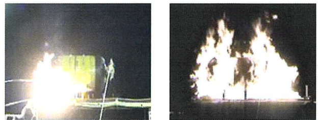
Fig. 26 Bonfire Test (Left: Localized Fire Test, Right: Engulfing Fire Test)
