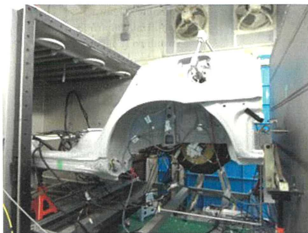
Fig. 27 External Appearance of Hydrogen Gas Pressure Cycle Test
