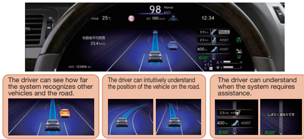
Fig. 10 Intuitive and Easy-to-Read Instrument Cluster Display
