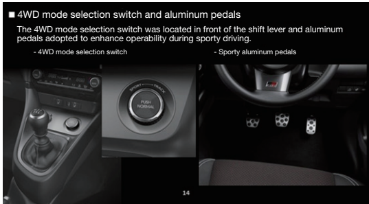
Fig. 16 4WD Mode Selection Switch and Sporty Aluminum Pedals
