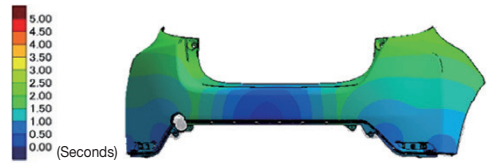
Fig. 13 CAE Flow Analysis for Rear Bumper
