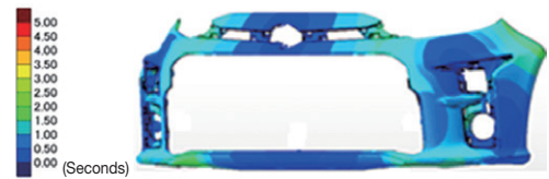
Fig. 12 CAE Flow Analysis for Front Bumper
