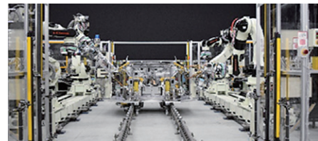
Photo 3 Completion of Spot Welding Using Single Jig (General-Purpose Cell)
