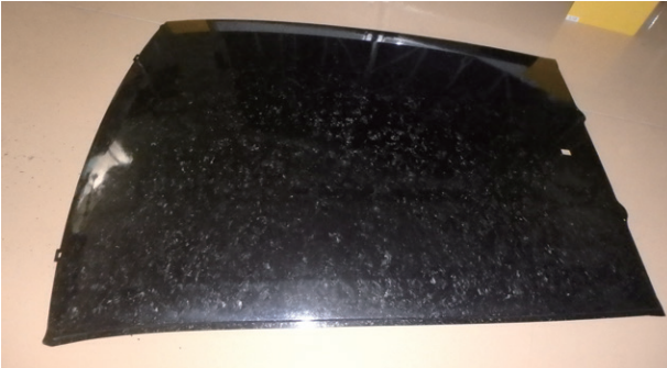
Fig. 6 CFRP Roof Panel
