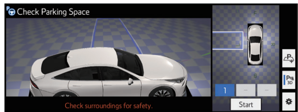
Fig. 14 Display of Parking Space in Memory Function
