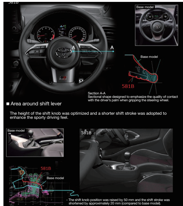
Fig. 15 Dedicated Steering Wheel and Optimization in Area around Shift Lever
