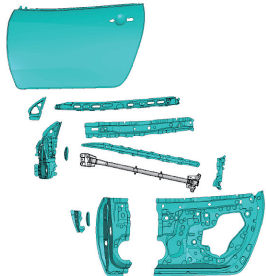
Fig. 4 Aluminum Side Door Components (Highlighted in Light Blue)
