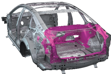
Fig. 10 Annular (Ring-Shaped) Structure to Enhance Rear Rigidity
