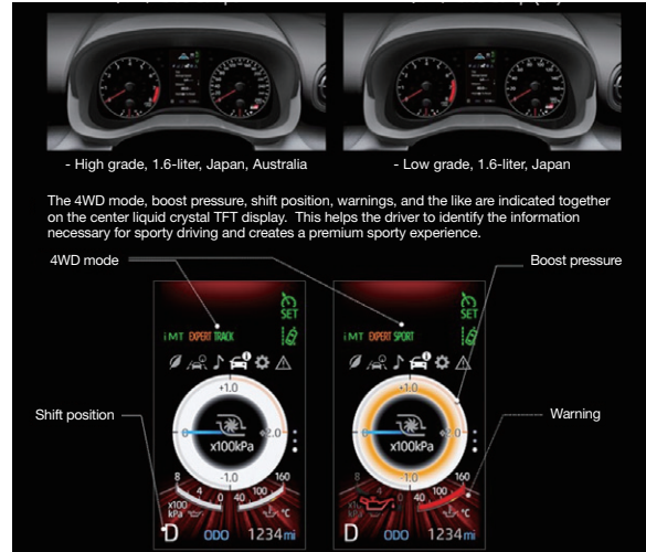
Fig. 14 Analog Meter Cluster and Liquid Crystal TFT Display
