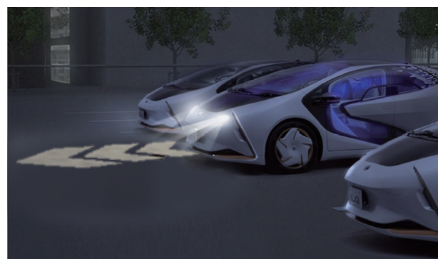
Fig. 15 Illustration of Notification when Vehicle Moves Off
