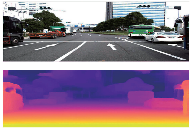
Fig. 6 Inferring Depth from Monocular Vision to Help Reduce Requirements for Expensive Lidar Scanners, Top: Traffic Scene in Odaiba, Bottom: Depth Inferred by the Network (Yellow Means Close and Violet Means Far Away) (3)
