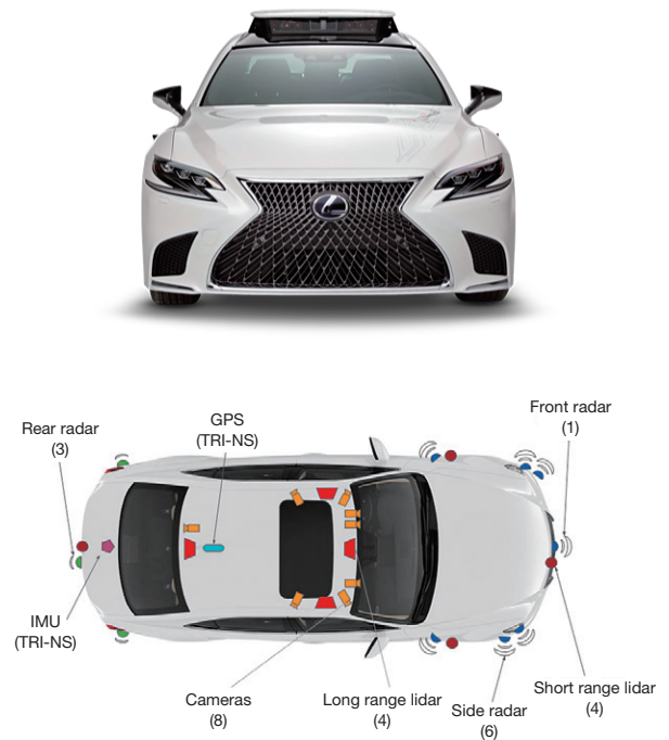
Fig. 3 The Sensor Configuration of the P4 Including an Array of Advanced Camera, Lidar, Radar and Navigation Sensors, Combined with Powerful Onboard Computation
