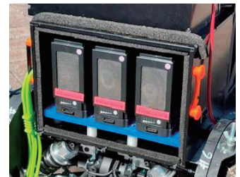
Fig. 6 Internal View of Battery Box
