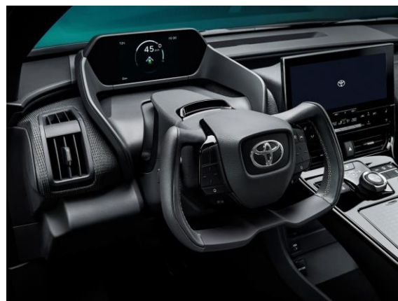
Fig. 12 Model Equipped with Steer-by-Wire System and Uniquely Shaped Steering Wheel
