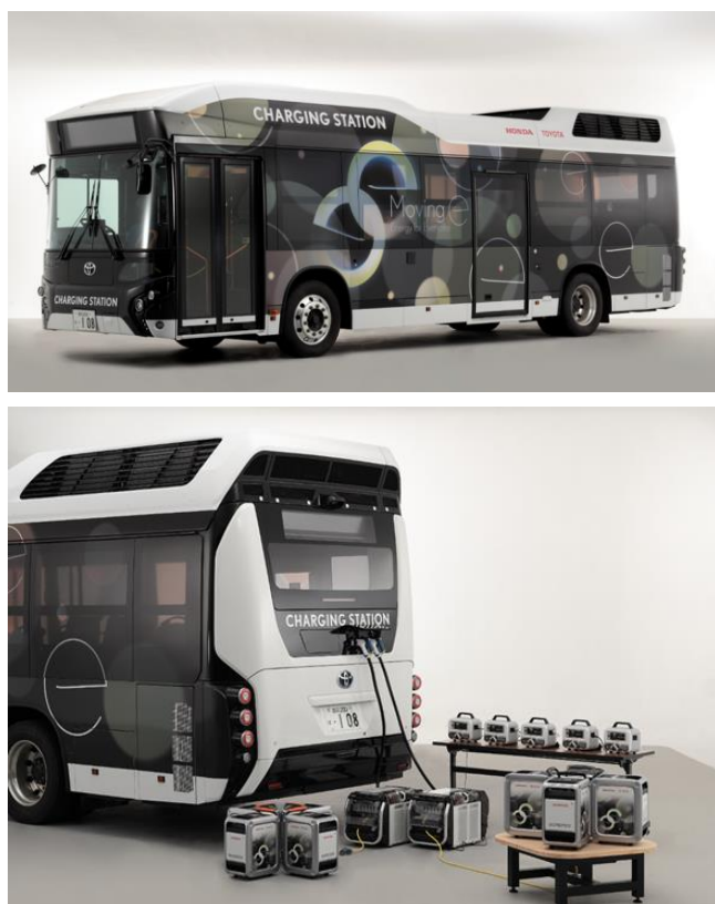
Fig. 45 Charging Station FC Bus
