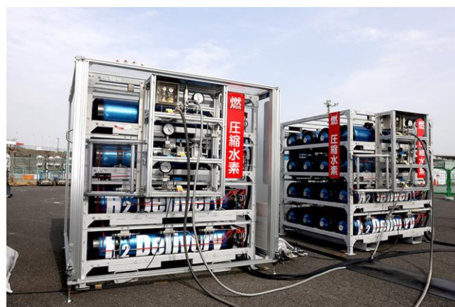
Fig. 32 Hydrogen Curdle Containing Resin High-Pressure Hydrogen Tanks
