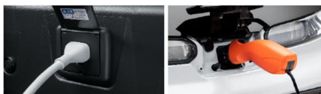
AC 100 V outlet (below passenger seat)
