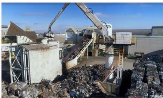
Fig. 7 Shredding of Crushed Vehicle Bodies
