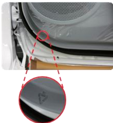
Fig. 5 Marking to Improve Dismantling Process of Door Trim
