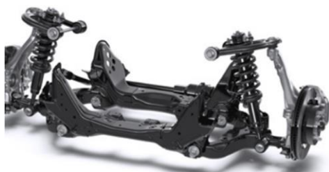
Fig. 8 High-Mount Double Wishbone Front Suspension
