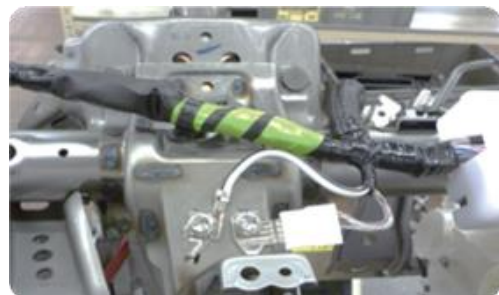
Fig. 8 Tape to Raise Visibility for Wire Harness Dismantling
