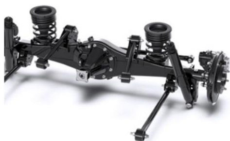
Fig. 9 Trailing Link Axle Rear Suspension
