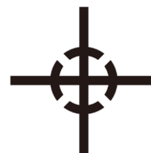
Fig. 2 Marking Indicating the Center of Gravity
