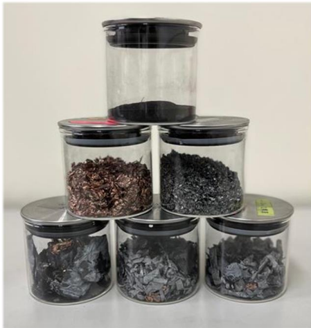
Fig. 11 Battery after Crushing and Separation
