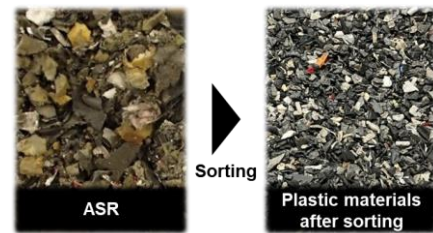
Fig. 14 ASR before and after Sorting
