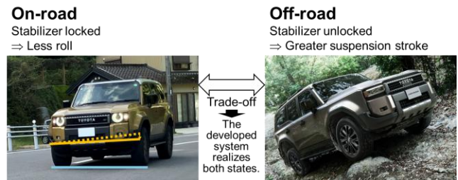
Fig. 1 Stabilizer Lock State on Different Road Surfaces
