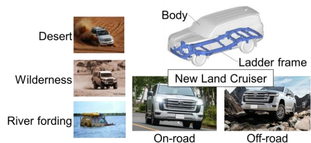
Fig. 1 Ladder Frame SUV
