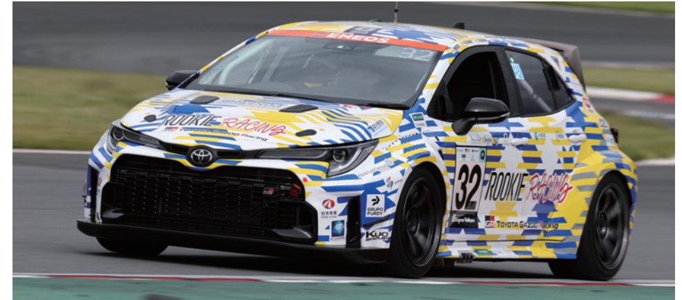
ORC ROOKIE GR Corolla H2 Concept with liquid hydrogen-powered engine
