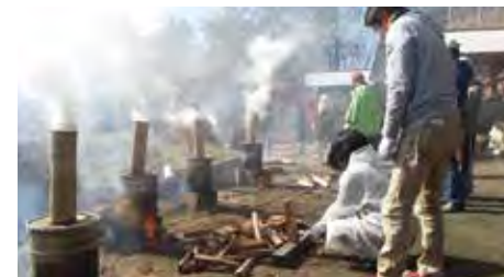
Bamboo charcoal making using pail cans
