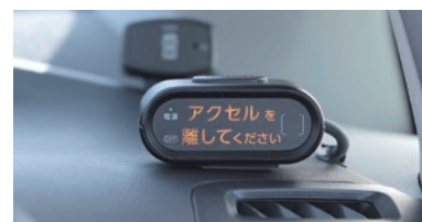
Display of the pedal misapplication prevention system for retrofitting
