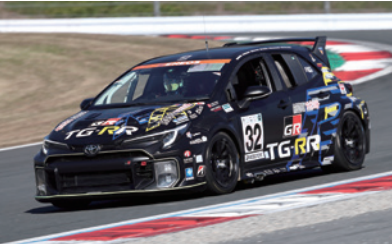
The GR Corolla with a liquid hydrogen engine
