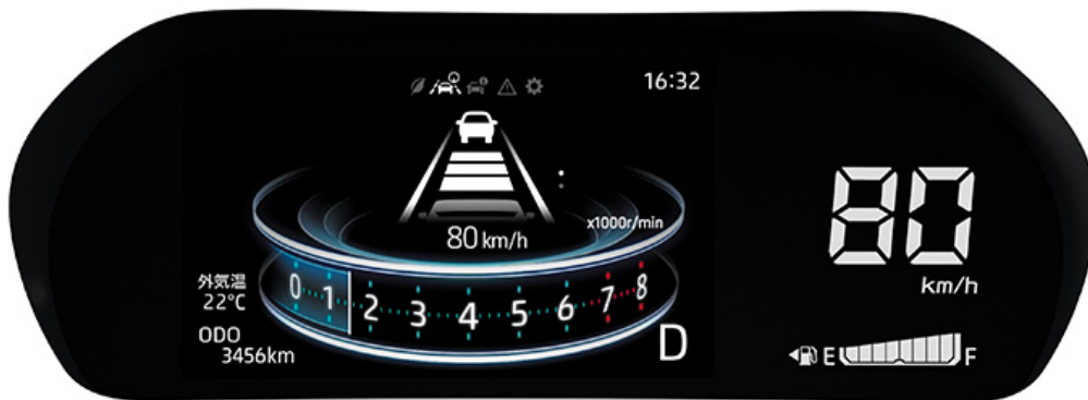
The seven-inch TFT color LCD display in the Advanced display mode
