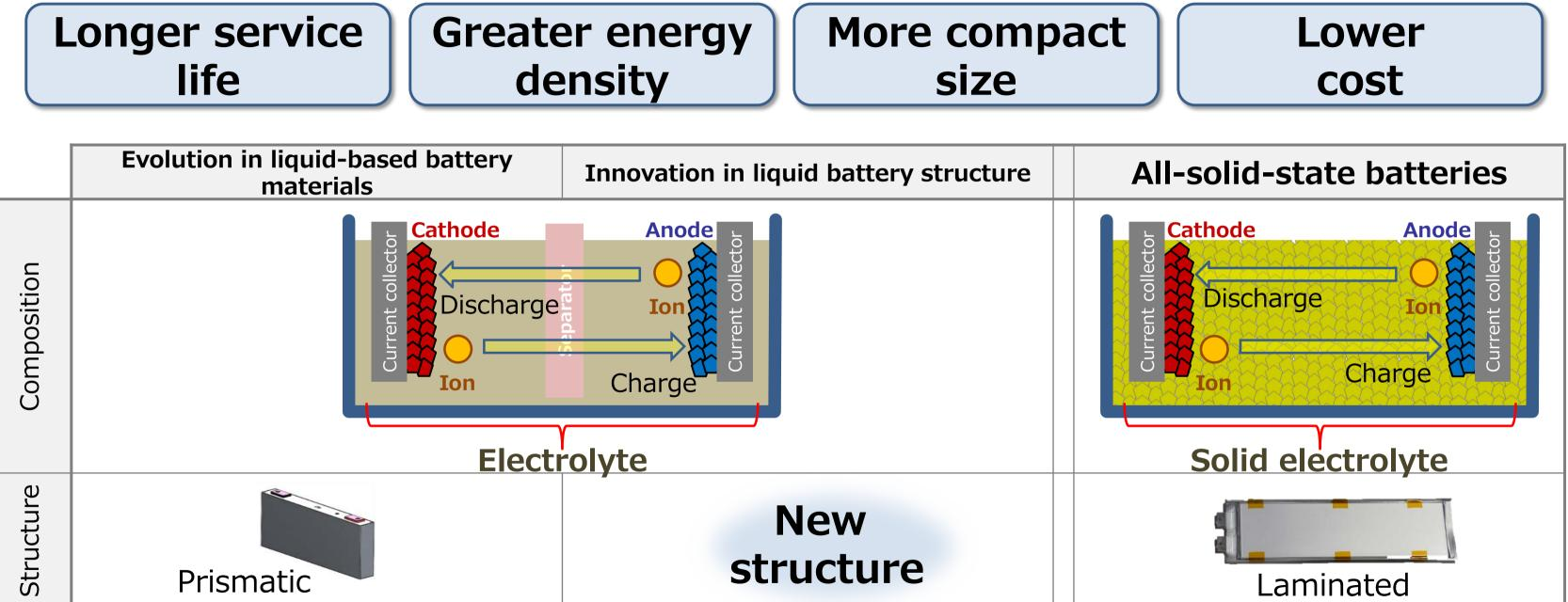
Taking on the challenge of developing a wide range of batteries for the second half of the 2020s Providing BEVs equipped with batteries with improved characteristics that enable driving with peace of mind
