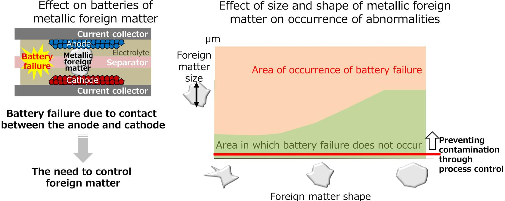
Determining the size and shape of foreign matter that can cause battery abnormalities and controlling the effect of foreign matter
