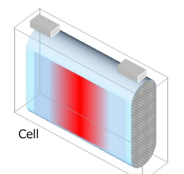
Simulated experiments to measure polarization of electrolyte components (which generates heat) during charging and discharging
