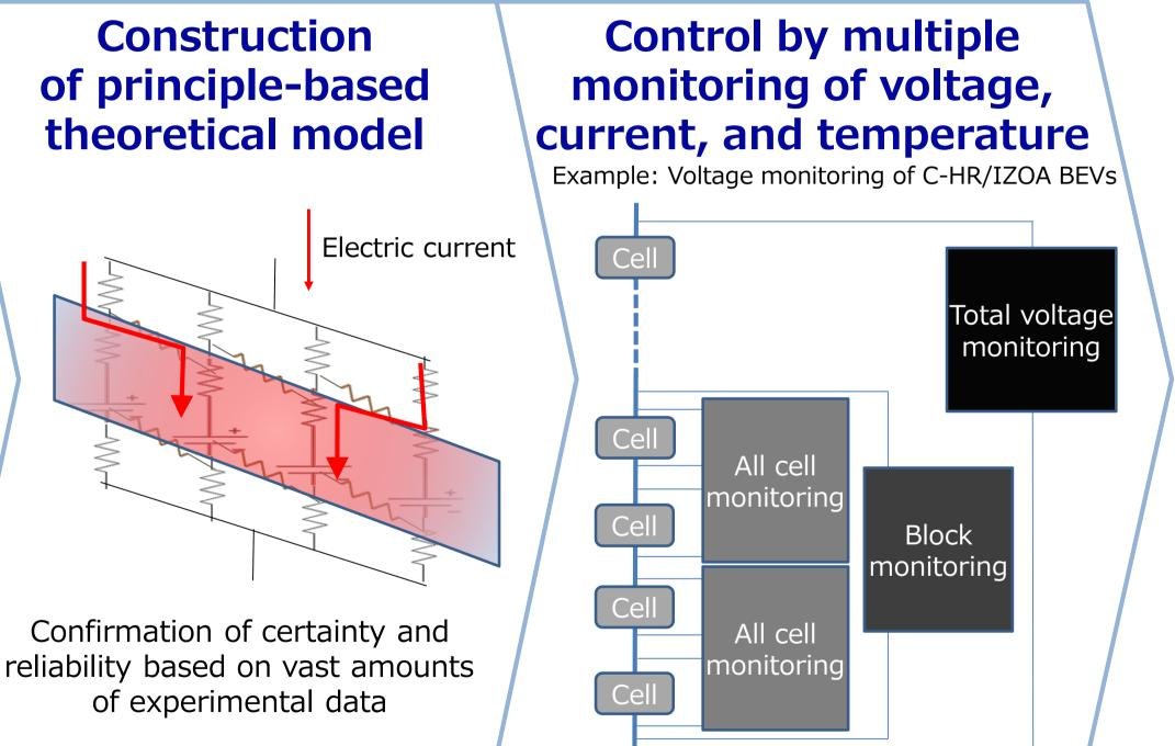
Multiple monitoring of voltage, current, and temperature to detect signs of and prevent abnormal heat
