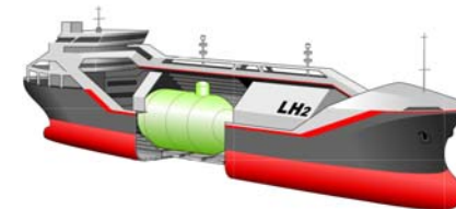
Liquid hydrogen transported by a carrier ship with highly insulated tanks
